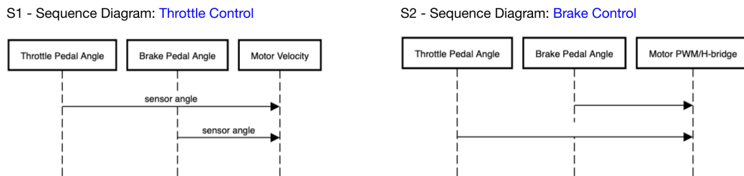
Figure 2: Sequence Diagram for Throttle Control (left) and Brake Control (right)
